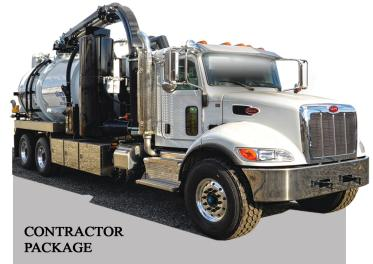
Vacuum Pump: 4,500 CFM 18" Hg Water Pump: 19 GPM 2,900 PSI Rear-mounted 25' boom with 270 degree rotation
